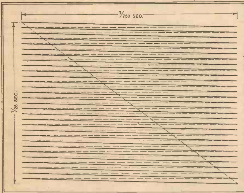
Fig. 28.—Television scanning in a cathode ray tube by two saw-tooth voltages.
