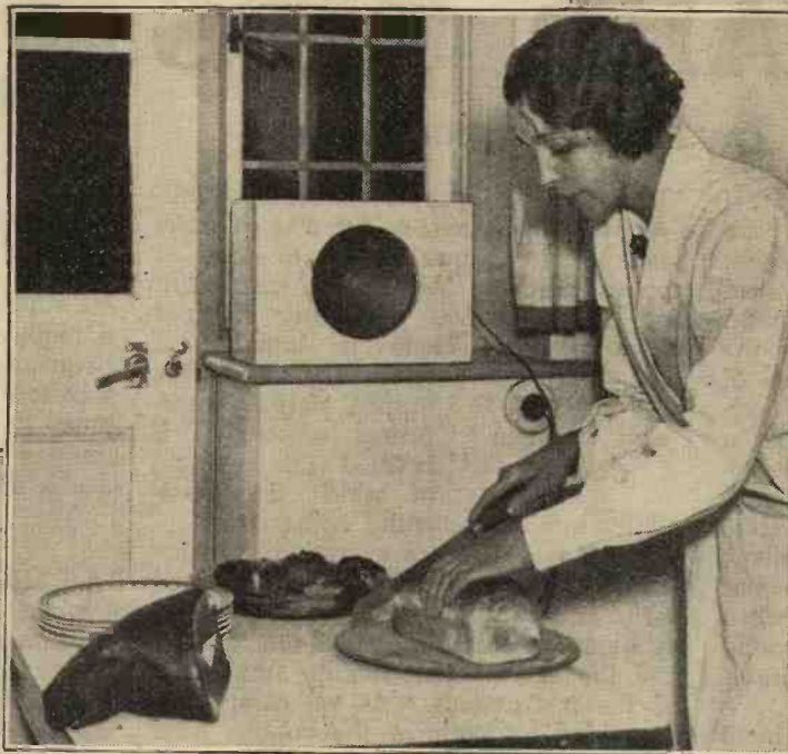
Appropriate loud-speaker mountings have been devised for each room. These photographs show (left) the bathroom speaker, protected from steam; (above) a white cellulosed cabinet for the kitchen, and (right) a practical form of mounting above a built-in bedroom cupboard.
