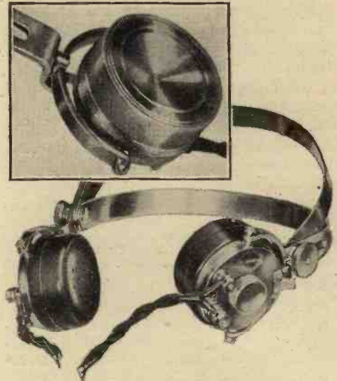
Brown's "A" type headphone, incorporating a cone diaphragm and an adjustable reed.
