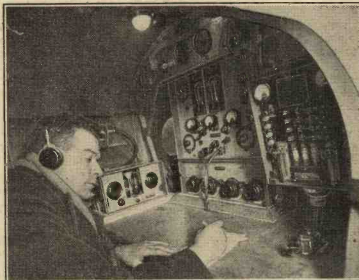
RADIO ON TRANS-PACIFIC FLIGHT. Captain C. T. P. Ulm in the Airspeed "Envoy" in which he will attempt a flight from Vancouver to Melbourne. The apparatus shown is (left to right) the Marconi "homing" device, Marconi medium- and short-wave transmitter (above) and receiver, and the switchboard for wireless and lighting current, which is derived from a wind-driven generator.
