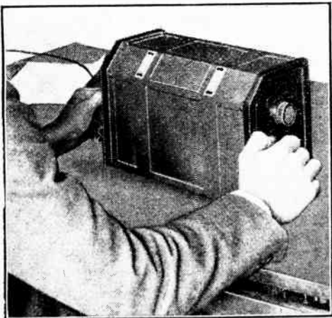
An early type of receiver with side knobs, allowing a natural and comfortable operating position.
