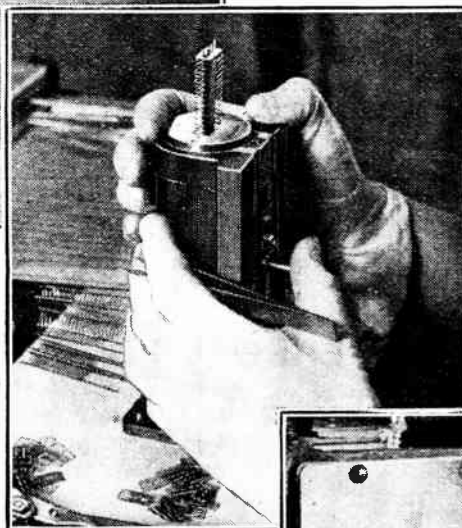
Above: How the cathodes are sprayed in Osram "Catkin" A.C. valves. Right: One of the jigs used to ensure accuracy of spacing in assembling the electrodes.
