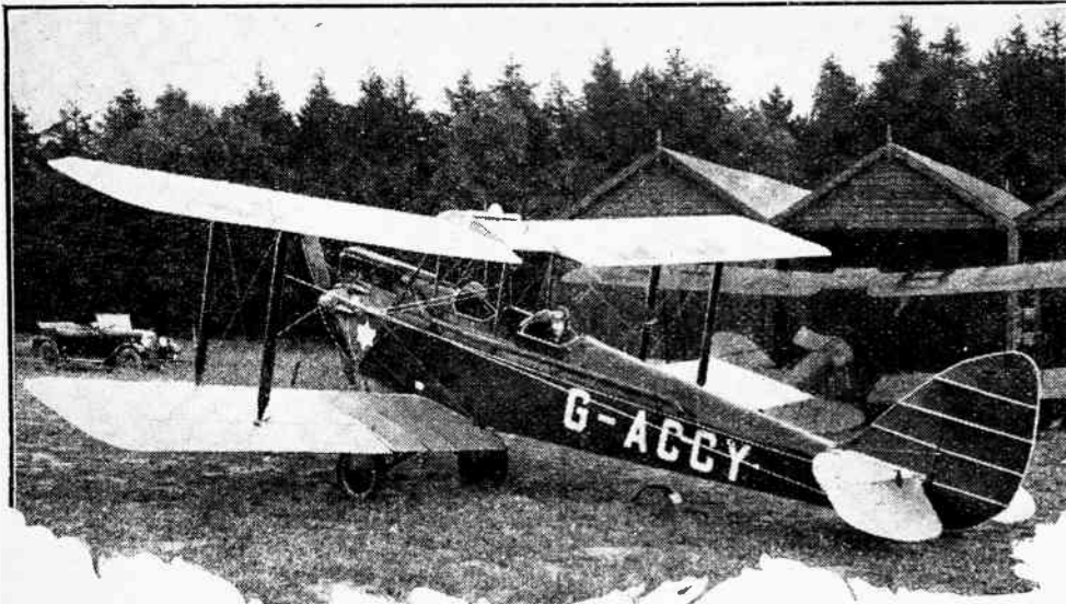
The Gypsy Moth ready for the start. The aerial can be seen slung between the left rear strut and the tail plane.
