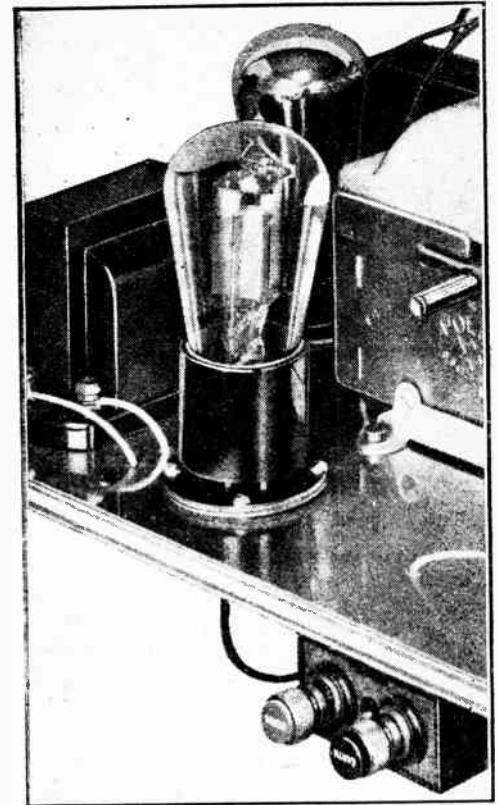
Showing the output circuit of "The Wireless World" Class "B" Ferrocart receiver, which delivers about 2 watts speech.
