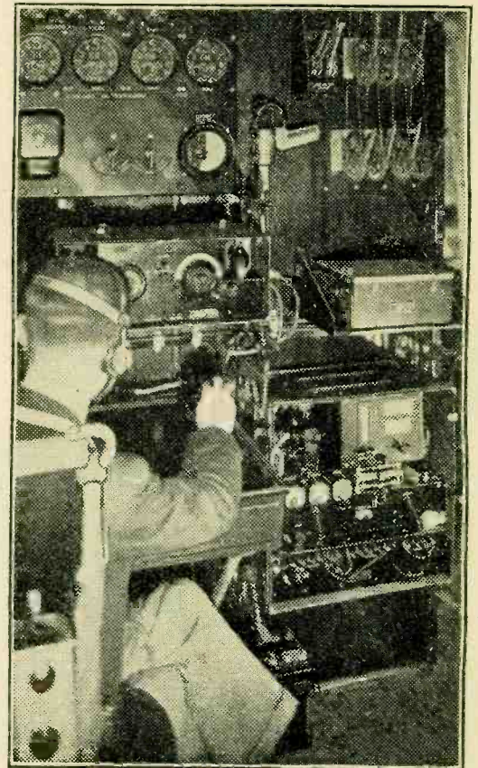
A typical passenger aircraft radio installation. The photograph was taken on one of the "Kent" type flying boats used on the Indian and African air routes.
