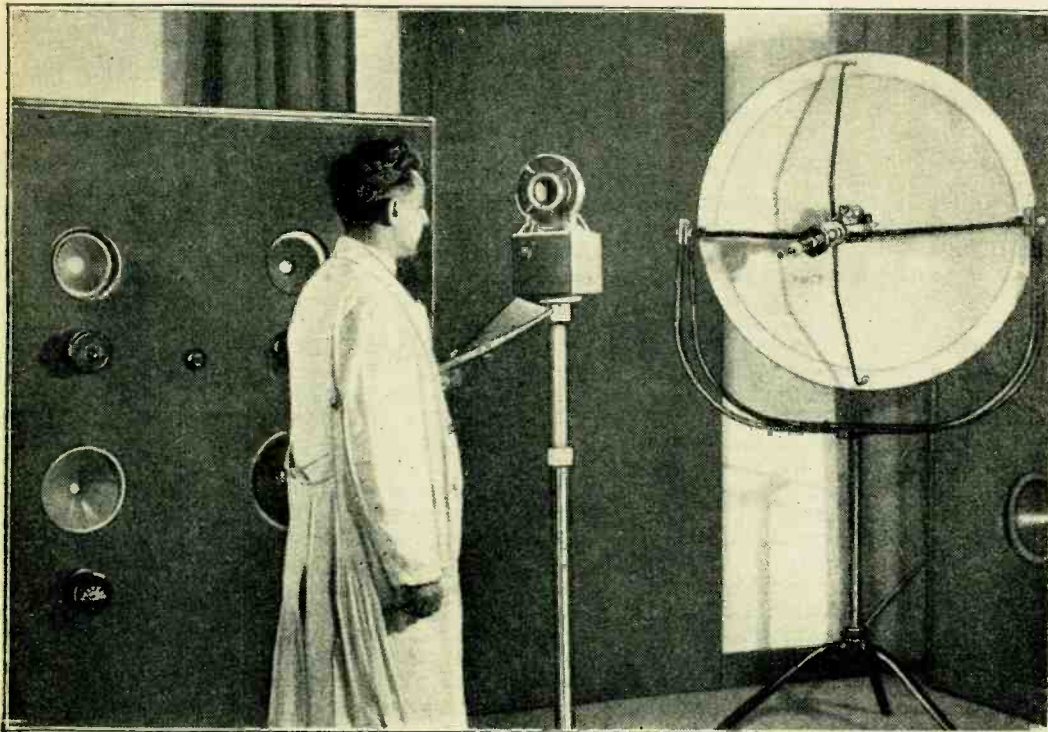
Radio research workers on the Continent are paying special attention to the problems of microphone and loud speaker design. The "soup-ladle" reflector on the right is a modification of the design which has become so popular in America. The microphone is a new condenser type which can be tested in conjunction with the various loud speakers seen on the left.
