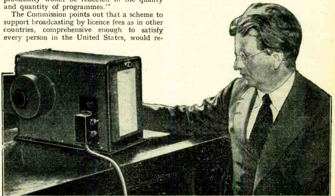
TELEVISION FOR THE HOME CIRCLE. Mr. John L. Baird photographed last week with the new home televisor in which the image is projected on a screen and is visible all over a large room.
