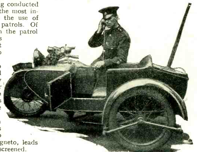
WITHOUT LEAVING THE SADDLE. A relay-actuated light device indicates to the patrolman that the headquarters transmitter is in operation.
