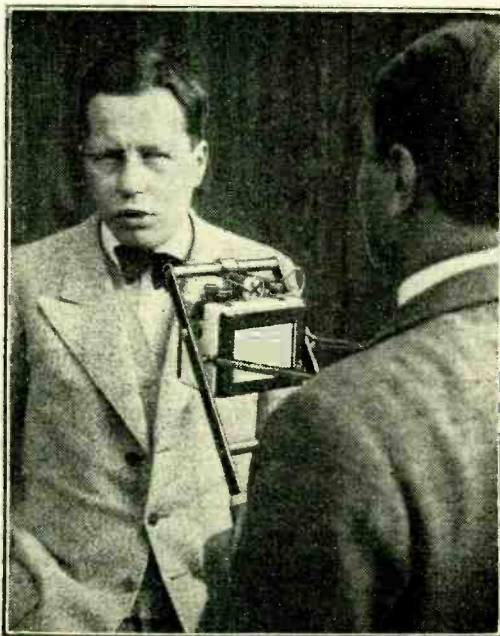
THE BROADCAST INTERVIEWER. A specially slung double-faced microphone used for radio interviews in Germany. The little black cross above the microphone face indicates that the circuit is "alive."
