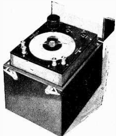
Sullivan simple capacity test set covering a range of 0.00005 mfd. to 1 mfd. with calibrated scale.
