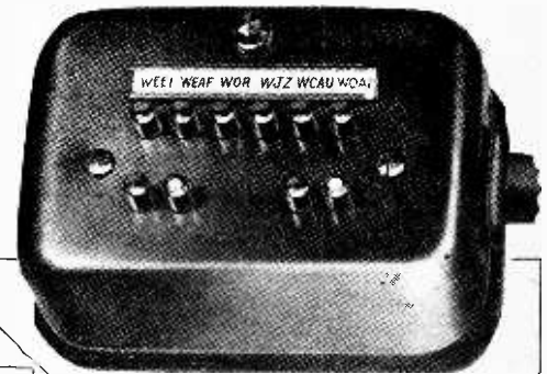
Fig. 1 (b).—Remote control unit and circuit arrangement for the device which can be attached to the Westinghouse and Radiola receivers.
