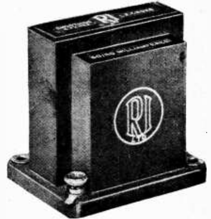
General purpose L.F. choke to carry 60 mA. of D.C. The rated inductance is 25 henrys. An R.I. product.
