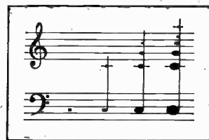
Fig. 15.—Overtones generated in the ear as the bass C is sounded more and more loudly. The sizes of the notes indicate roughly their intensity.
