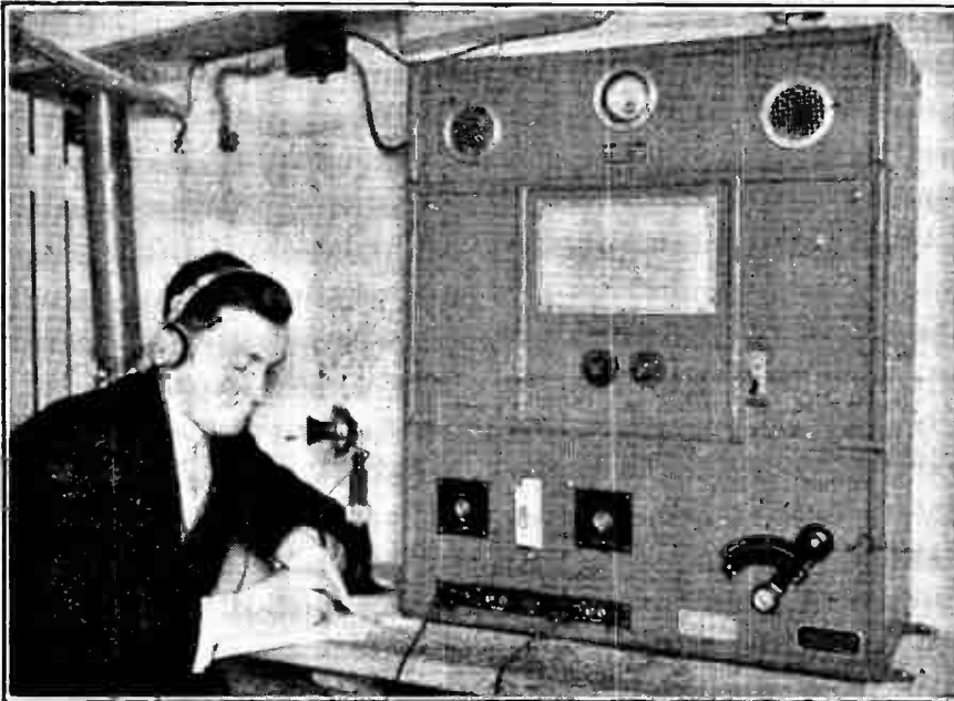
FOR THE WORLD'S FASTEST LIFEBOAT. —The totally enclosed wireless telephony transmitter and receiver installed by the Marconi Company in the new Dover lifeboat, the fastest in existence. Known as the type XMB.1., the set uses a transmitting power of 100 watts on a wavelength of 900 metres, and is designed for work under the roughest conditions. The lifeboat is specially equipped for aircraft rescue work,
