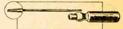
"Nipsit" screwdriver, showing blade removed from holder and enlarged view of split end.
