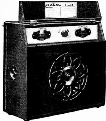
The edgewise drum tuning dials set in the narrow white panel give a distinctive appearance to the Marconiphone Model 53 portable.
