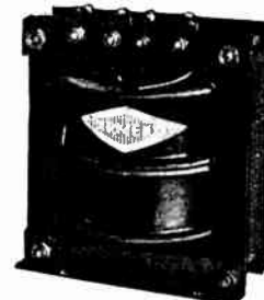
PARMEKO DOUBLE CHOKE Inductance 80 henries. Current carrying capacity of windings, 50 milliamps. Resistance 475 ohms.
