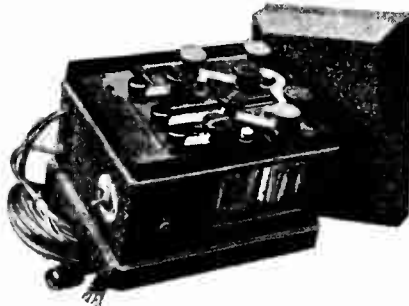
Oldham "Auto-Power" unit with self-contained battery and Balkite charger for supplying L.T. current.
