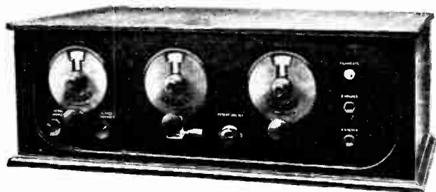
Two views of the Igranite H.F. set, which covers all the ultra-short wave bands.
