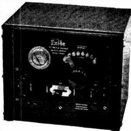
Exide H.T. trickle charger with variable output up to 50 milliamperes.
