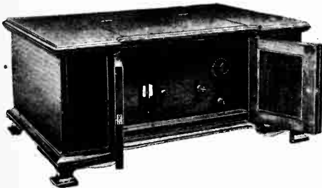
A Gambrel A.C. mains set with screened grid H.F. amplifier and a single finger tuning control.
