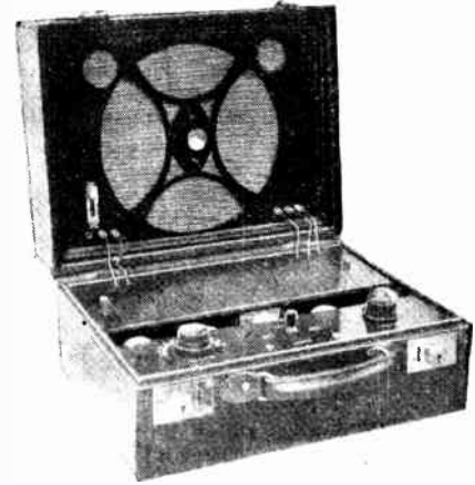
Burgoyne suitcase portable 5-valve receiver. Provision is made for using a gramophone pick-up.
