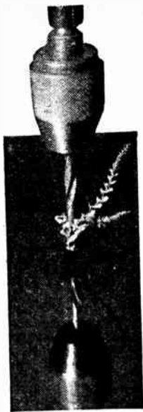
Drilling "Resiston" is simple. The long, unbroken "chips" curl away from the drill point, leaving a clean hole free from ragged edges or cracks.
