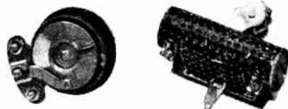
The Royal-Frost Gem rheostat and the Electrad Truvolt variable high resistance unit. (Rothermel.)
