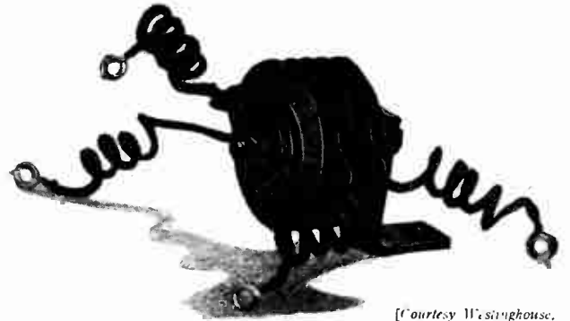
Fig. 2.—A typical metal-oxide rectifier unit assembled.
