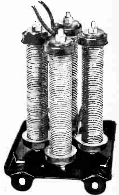
Fig. 5.—Showing the construction of a Westinghouse high-voltage rectifier for an H.T. battery eliminator.
