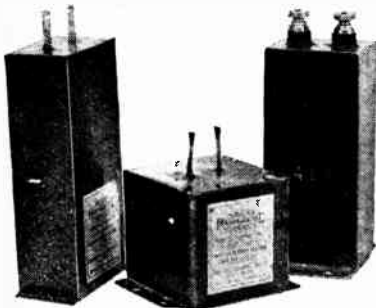
(Above) Dubilier electrolytic condensers of over 1,000 mfd. capacity, compared with a standard 2 mfd. condenser, and with
