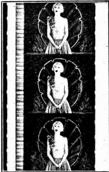
Fig. 1.—A specimen of film on which sound has been photographically recorded on the left-hand side.
