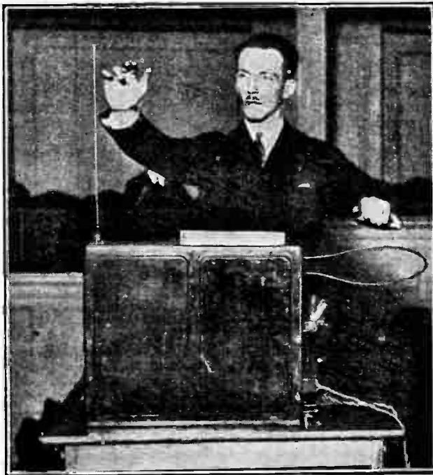
Prof. Theremin with his apparatus; the vertical rod on the left influences the pitch of sound produced, while the loop on the right controls volume.
