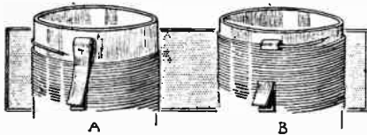
Fig. 2.—Securing the last turn of a solenoid coil by means of a short length of tape.
