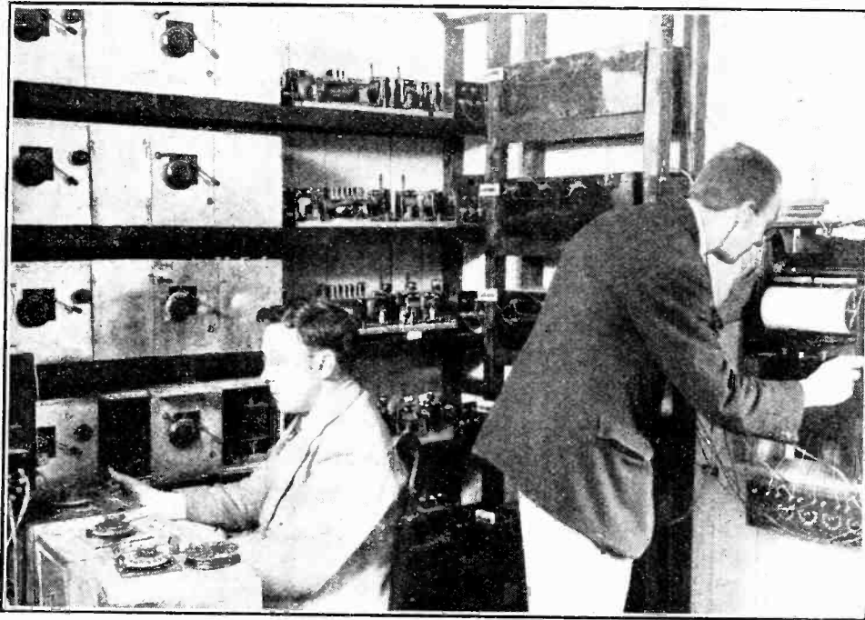
Fig. 4.—Apparatus for recording atmospherics simultaneously on six different wavelengths. There are nine valves in each of the six receivers.
