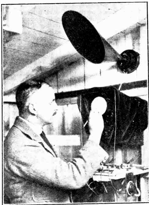
Fig. 3.—Visual direction-finder. The observer is watching the fluorescent screen upon which the direction of the atmospheric is indicated by a line of green light.
