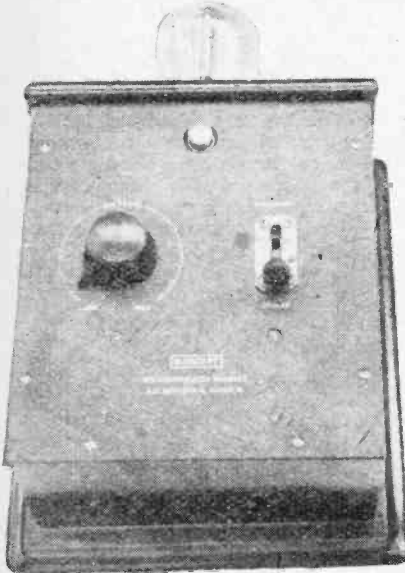
Burndept H.T. accumulator charger for use on A.C. supply. The charging rate is regulated by the filament brightness and is indicated by means of a glow lamp.
