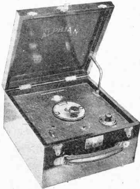
The Alphan station tuner. A heterodyne wavemeter for use in broadcast reception.
