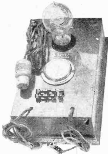
Liberty testing set for voltage determinations, insulation and continuity tests.
