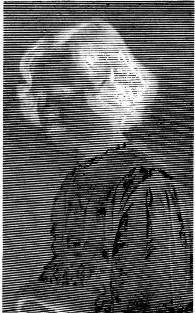
THE IMAGE AS PREPARED FOR THE TRANSMITTER. The cross-lines, produced by photographing through a ruled screen, are composed of a hard non-conducting film.
