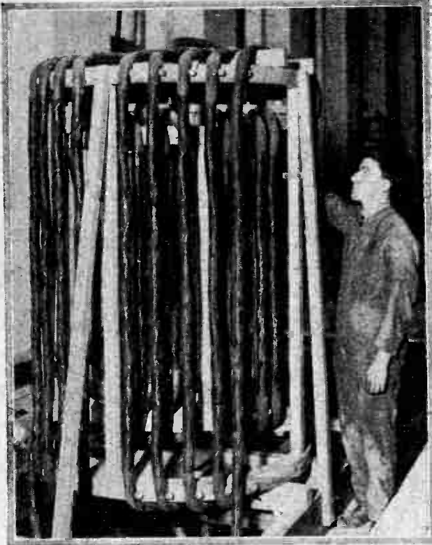
ONE OF THE TUNING VARIOMETERS. It is built entirely on a wooden frame work and the cable consists of 6,561 strands of No. 36 S.W.G. enamelled wire.
