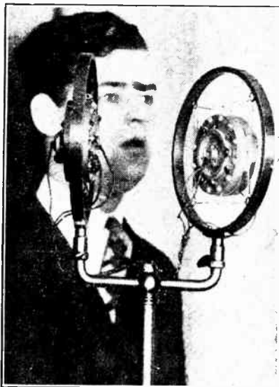
A TWIN MICROPHONE. A novel form of double microphone which has made its appearance in America. It is designed to give extreme sensitivity over a wide range of frequencies.
