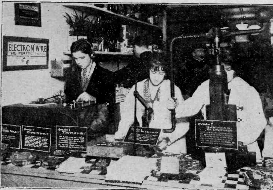
Making and testing Thera condensers at the stand of the Sel-Ezi Wireless Supply Co., Ltd. The testing equipment is supplied by Faraday House.
