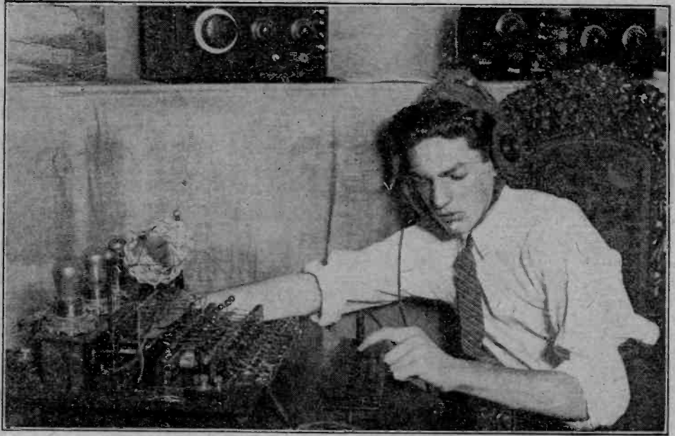
Automatically tuned receiver entered in the competition for amateur constructors. By means of a series of push switches and magnetic relays any one of a series of broadcasting stations may be selected.
