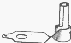
The one-piece valve socket, spring and tag used in the construction of Benjamin valve holders.
