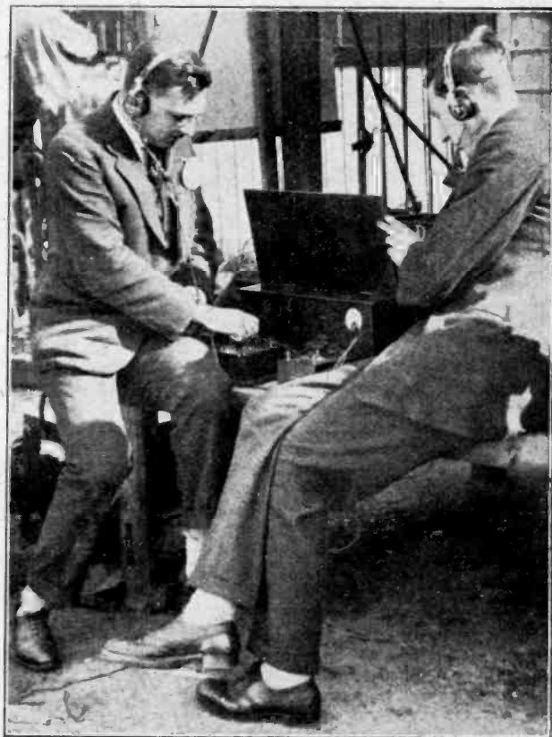
Ca-ptain West, Chief of the B.B.C. Research Department, regu-lating one of the potentiometers used to control the strength of the signal passed to the line circuit connected with Savoy Hill.
