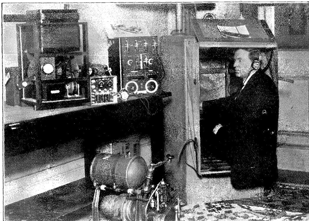
The new Marconi lifeboat set. Using a quenched spark transmitter, the installation has a range under normal conditions of 50 miles. The receiving gear includes a direction finder.
