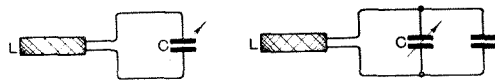
Fig. 2. A circuit consisting of a coil and a condenser only, and Fig. 3, a circuit with a coil, tuning condenser and a fixed condenser.
