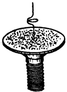
Fig. 3. The terminal head is covered with a piece of thin platinum foil for conducting experiments with amorphous powder detectors.
