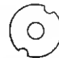
Fig. 10. Slotted washer for spacing winding cheeks. Two wires are wound on together to give a spaced spiral formation. The slots in the washer prevent irregular bends on the inner turns.
