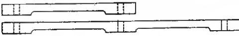
Fig. 3. Ebonite spacing strips. A hollow on the underside gives clearance to the windings.
