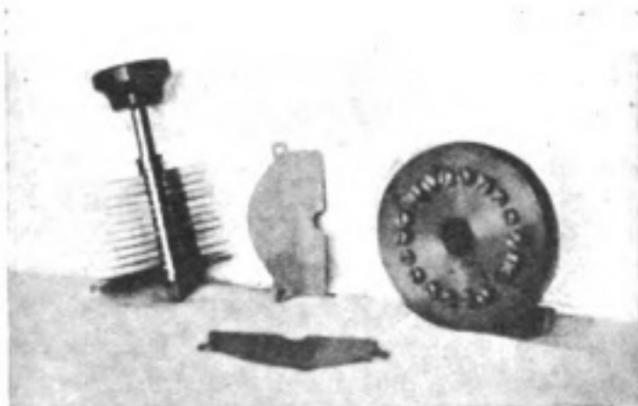
Fig. 1. Type of variable condenser used in C.W. and Spark Receiver.
