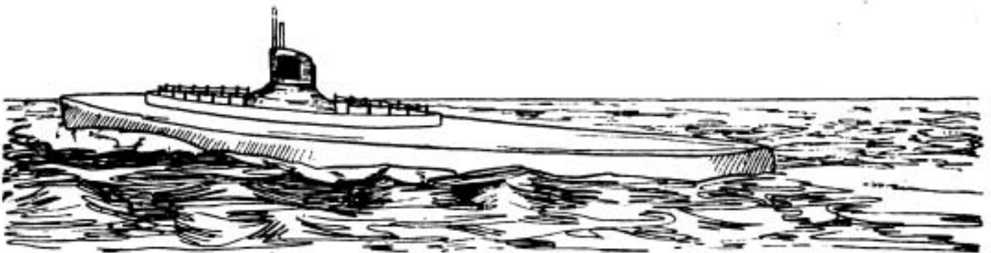
Fig. 2. Arrangement of fixed-frame Aerials on Submarine. (The frames containing the windings are mounted on each side of the conning tower. The position of one of them is indicated by the black square in this sketch.)
