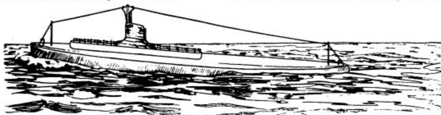
Fig. 3. Arrangement of single-turn loop Aerial on a Submarine. (The insulated wire is connected to the hull at both ends.)
