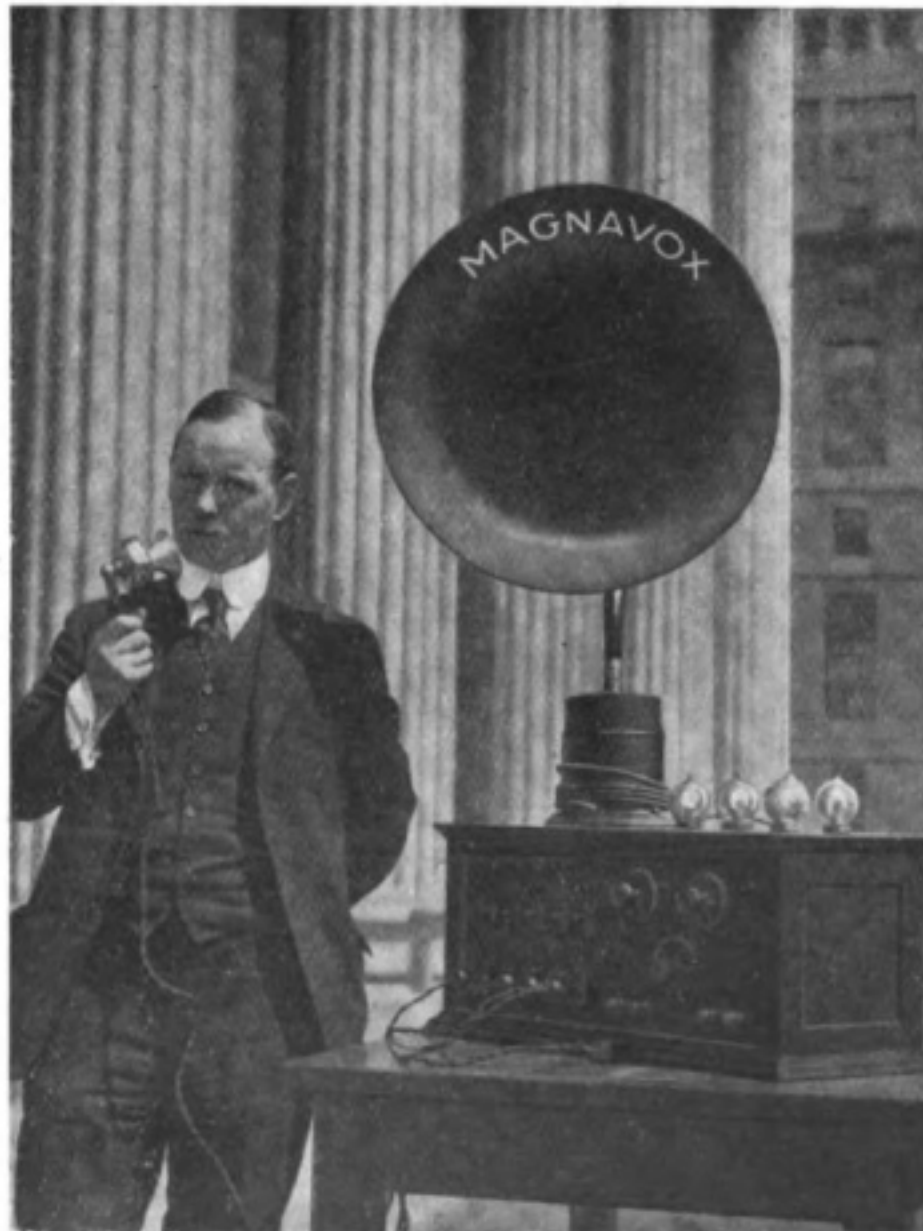
Photo Topical Press. The Magnavox, by means of which huge crowds heard President Wilson's Victory Loan appeal spoken by an aviator flying at a height of 3,000 feet.
