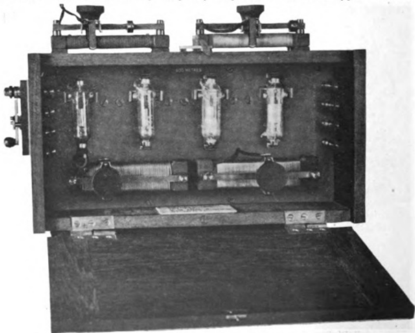
MARCONI VALVE AMPLIFIER AND DETECTOR, TYPE 50.
