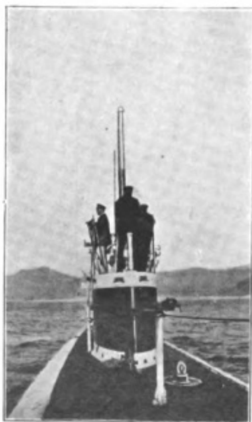
VIEW OF DECK AND CONNING TOWER LOOKING FORWARD. THE TELEPHONIC BUOY APPEARS IN THE FOREGROUND.
