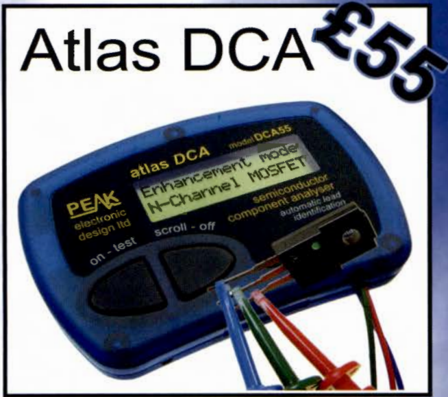
Atlas DCA - Model DCA55 Semiconductor Analyser
