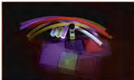
Polymer OLEDs are manufactured in solution (see bottle) but can be deposited onto various shapes (see tubes and plates). These samples are photoluminescing as a result of being illuminated by UV light
