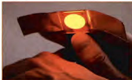
The polymer OLED device is printed onto a glass substrate which is then incorporated into a "bandage" structure for application to the patient's skin
