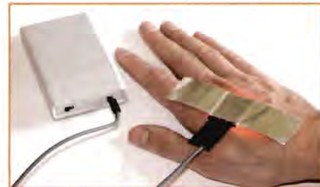
The polymer OLED bandage in use with its portable power supply
