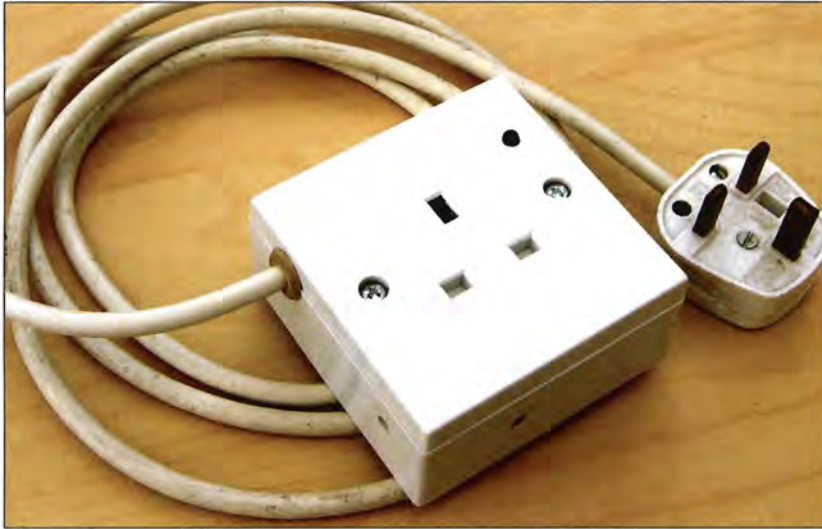
Standard plug-box, fitted with mains cable and plug, and with three holes cut for the dual colour indicator LED, access of light to the LDR and access to set up the light level at switch-on
