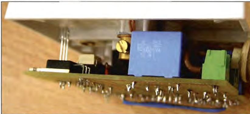
Edge view of completed PCB attached to the front face of the plug box
