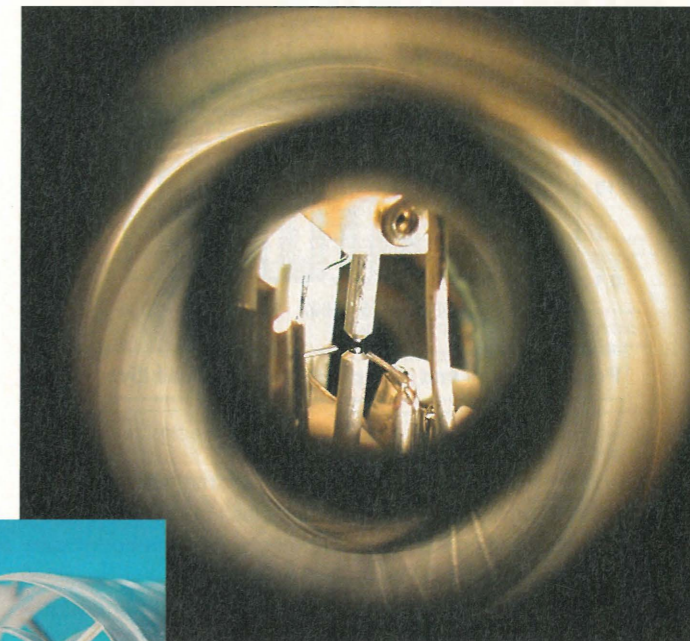
Above: The ovens and electrodes of the NPL strontium ion end-cap trap, viewed in situ in a vacuum chamber
