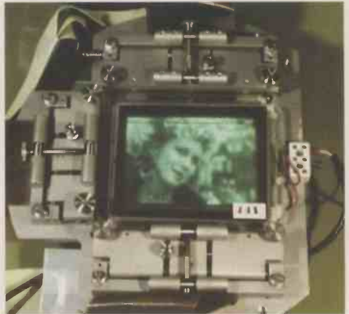
PFE proved its technology worked, with displays limited only by its rudimentary lab-based manufacturing equipment, it claimed. Now FEDCO aims to take it to production
