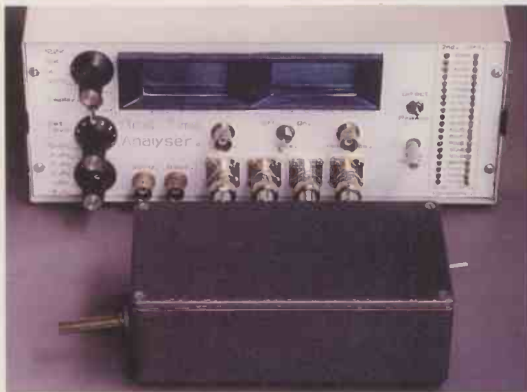
Fig. 2. The four BNC connectors mounted at 22mm centres, provide true four terminal measurements, isolating the test current from the voltage being measured. These enable a quick change from measuring capacitor distortions to evaluating low power amplifier circuits, simply by change of test jig as shown, with no change of the distortion meter internal circuitry.
