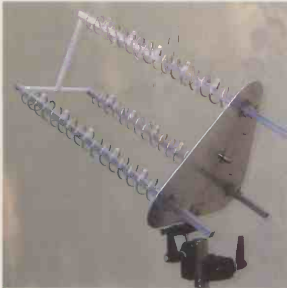
Fig. 9. TriHelix Antenna on the Support for AO40 Satellite Reception.
