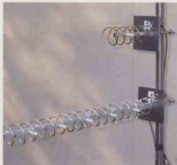
Fig. 8. Five Turns and 16.7 Turns Helices in Test.
