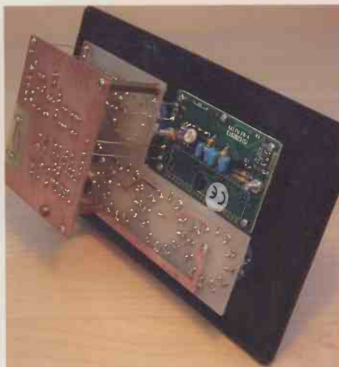
Completed project, showing the interconnections between the DVM and the two PCBs.
