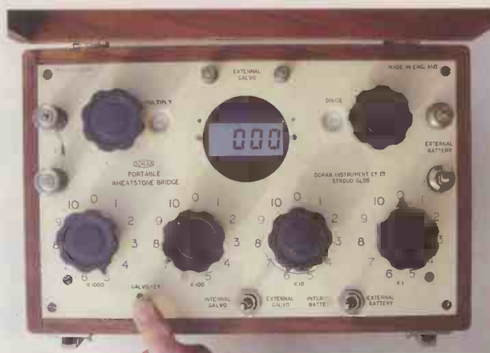
The original Wheatstone bridge with the galvanometer replaced with a DVM. Balance is achieved with a 5.6kΩ resistor.
