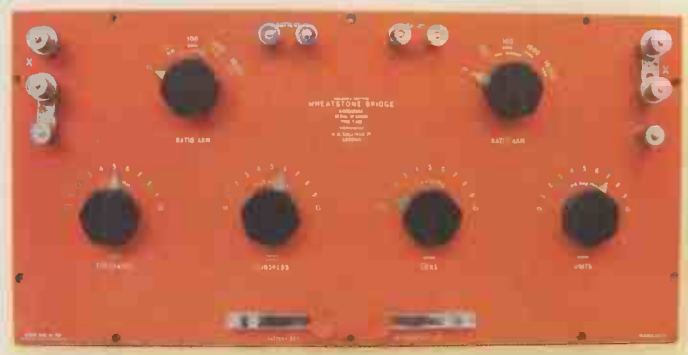
An original Wheatstone bridge, without galvanometer.
