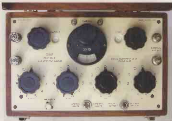
An original Wheatstone bridge, fitted with an integral galvanometer.
