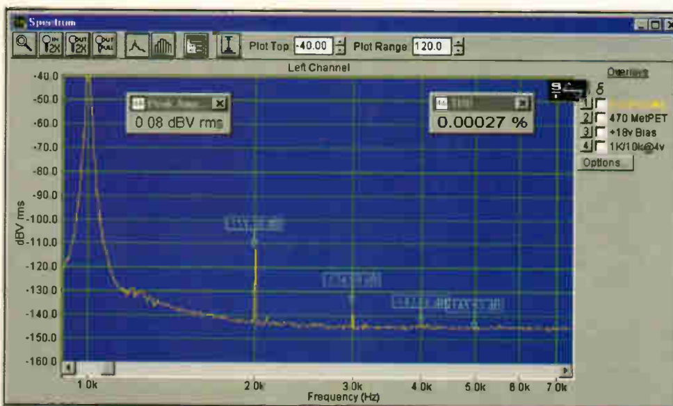
Figure 4: With no bias, this exceptionally good 0.1µF 63 volt type 470 metallised PET capacitor from BC Components, with magnetic leadwires, measured just 0.00004% distortion. With 18 volts DC bias, the second harmonic increased 22dB from -133.3dB to -111.4dB (distortion increased six times.) Intermodulation products are just visible, either side of 2kHz.
