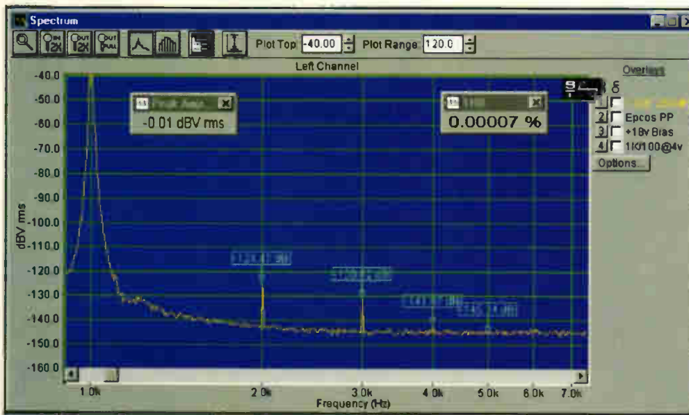
Figure 12: If you have room for a capacitor with 22mm lead spacing, this 1.0µF 250 volt Epcos with DC bias voltage, distorts less than most capacitors with no bias.
