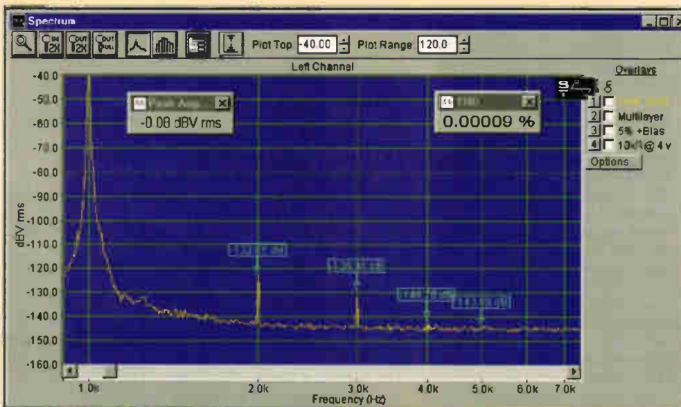
Figure 5: Distortion measurement of a Class 1 ceramic using 100Hz and 1kHz signals at 4 volts and 18 volt DC bias. With no bias this tiny 10nF 50 volt COG multilayer capacitor measured just 0.00006%. Second harmonic was -128.5dB, the other levels remained as shown.
