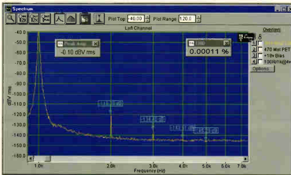
Figure 8: The first of two plots which explore the effect an increase in metallised PET film thickness might have on distortions. With no bias, distortion of this 100 volt capacitor measured 0.00006%, second harmonic -126.2dB. With DC bias, second harmonic increased by 7dB and distortion to 0.00011%
