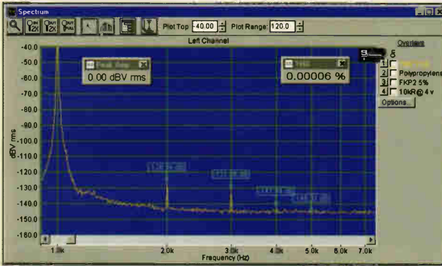
Figure 9: The small Wima FKP2 foil/Polypropylene capacitor shows similar performance except for 2dB increased second harmonic. Distortion just 0.00008% with 6 volts stimulus and 30 volts DC bias.
