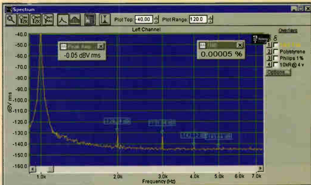
Figure 7: This now discontinued Philips extended foil/Polystyrene 1% axial lead capacitor, with 4 volt signals and 18 volt DC bias, shows negligible distortion. With test signals increased to 6 volt and DC bias to 30 volt second harmonic increased less than 4dB and distortion to 0.00007%.
