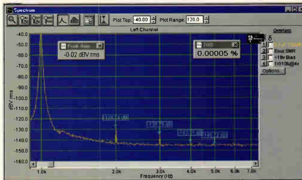
Figure 10: This 0.1 \mu F 100 volt Evox Rifa SMR capacitor, provides a superb low distortion performance with or without DC bias, even as high as 30 volts and no intermodulation products were seen.
