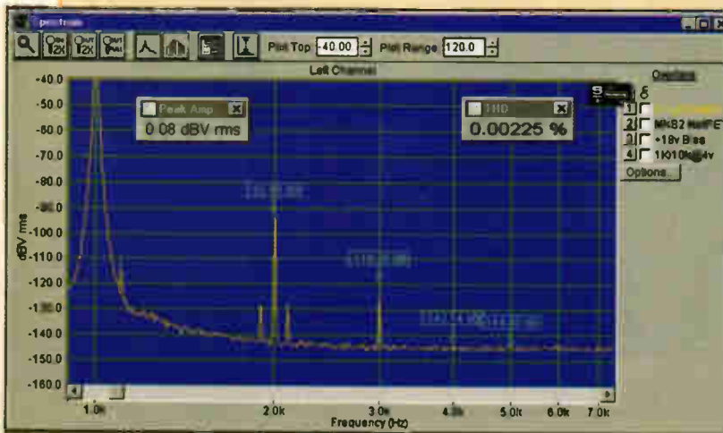
Figure 11: Tested with no bias, this 0.1µF MKS2 metallised PET capacitor measured 0.00016% with clearly visible intermodulation products. With 1B volts DC bias, the second harmonic increased dramatically, from -119.0dB to -92.9dB and harmonic distortion to 0.00225%.
