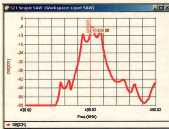
Figure 5: Effect of inductive mismatch on bandpass
