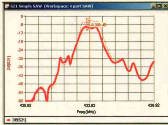
Figure 6: Effect of capacitive mismatch on bandpass
