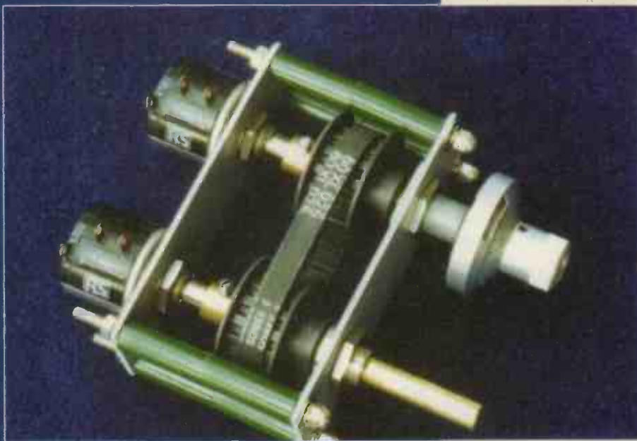
Fig. 1. This semi-overhead view of my dual gang version, illustrates both types of outrigger bearing. Clearly shown is the possibility of reducing the depth needed for all three assemblies. Unwanted spindle length will be removed at final installation. For this assembly, the potentiometer spindles were spaced on 40.5mm centres. This spacing provided easy connections to my circuit board.
