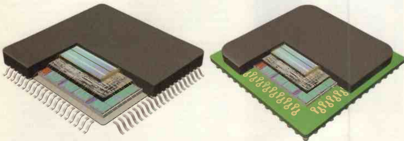
A thin film substrate for stacking multiple die in a package has been developed by Swedish firm Strand Interconnect. In order to avoid thermal expansion problems, the interposer material is made from silicon.
