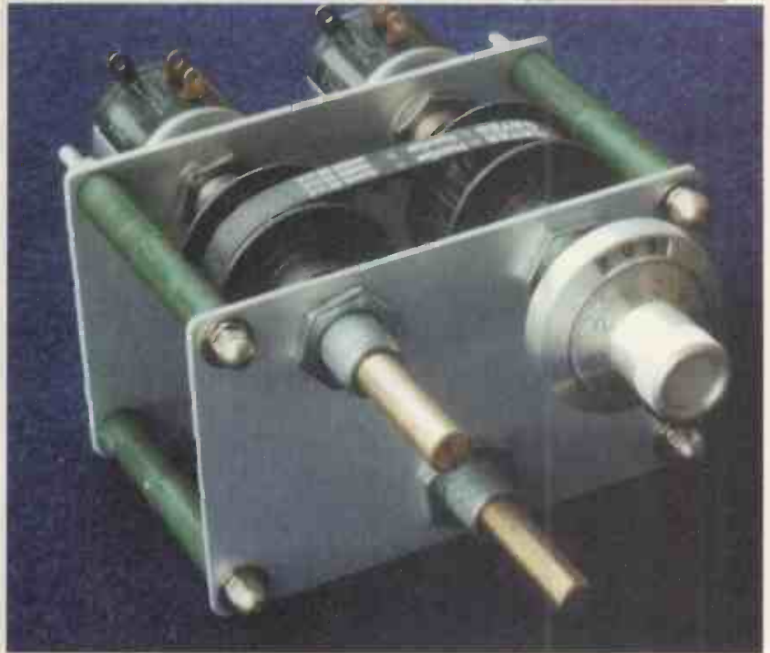
Fig. 2. This triple gang version required care when marking out the drill centres for each potentiometer. Because of the 120° belt wrap-around, my original calculations resulted in too much tension in the belt. I found best results when the spindles were equi-spaced by 35.5mm, at the corners of an equilateral triangle.
