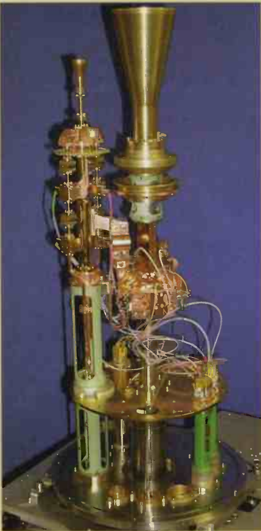
The Australia Telescope can now receive frequencies of up to 100GHz, following an upgrade with indium phosphide chips. Velocium, part of US electronics firm TRW, supplied the amplifiers and digital receivers. “The extremely high frequencies allow astronomers to take pictures of new phenomena with greater detail than ever before,” said Dwight Streit, boss of Velocium. The image shows one of the upgraded receivers.
