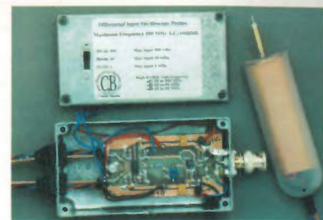
Fig. 10. Composite view of the prototype differential probes as tested. Both probes are housed in one half of a plastic traveller's toothbrush case. This has a wrap of copper foil inside to act as a Faraday shield. For ease of assembly the differential amplifier was housed in a 110 by 60 by 31 mm die-cast box. This PCB could easily fit in a much smaller box.
