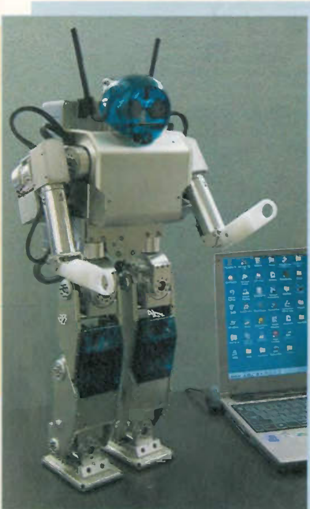
This very humanoid robot has gone on sale in Japan. Developed by Fujitsu, the HOAP-1 weighs 6kg and stands half a metre tall. It is aimed at development of motion control applications such as two legged walking. Fujitsu hopes to sell a hundred of the robots in the next three years – with the price described as 'open'.
