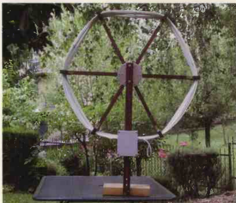
Fig. 10. A group of large coils that we used for the Q factor tests.
