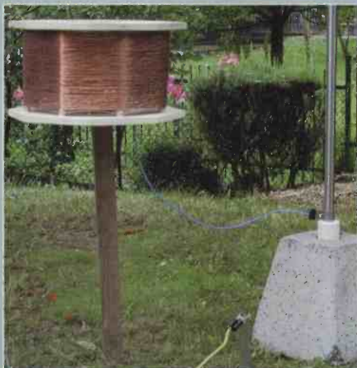
Fig. 1. At the base of the Marconi vertical antenna for 136kHz.
