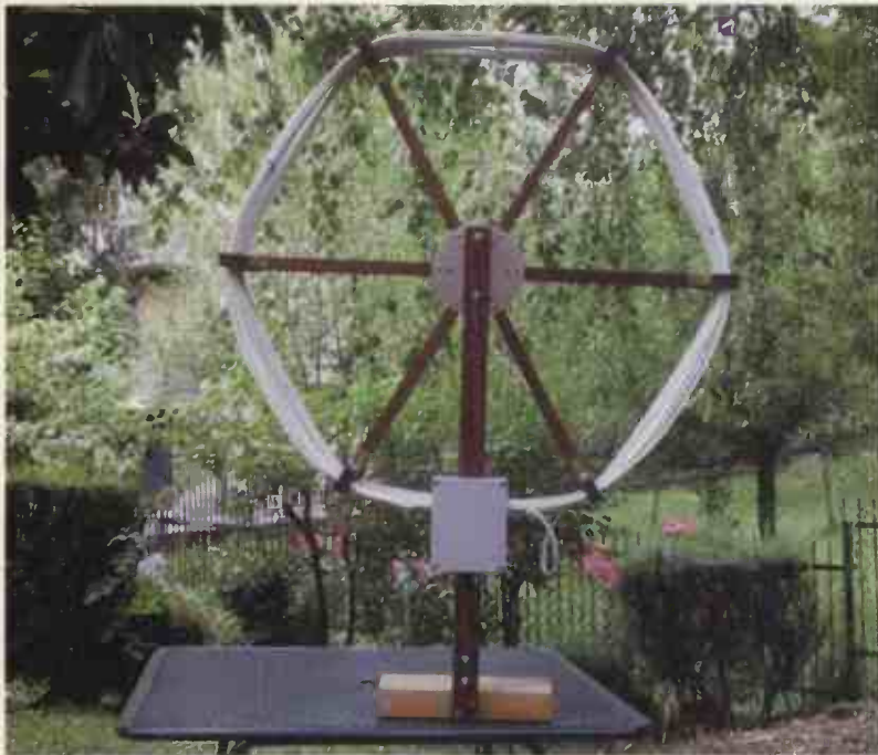
Fig. 12. Shielded and tuned LF loop antenna comprising 18 turns of TV-satellite cable, together with a balanced amplifier.
