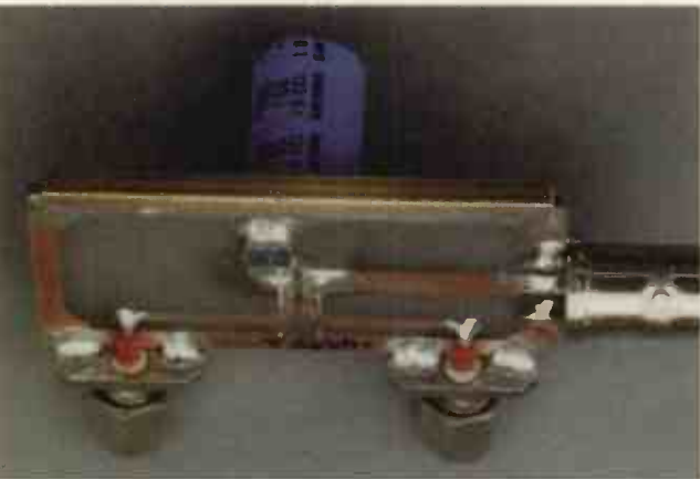
Fig. 7. Test jig specially developed for the |Z| meter differential voltage and phase measurements. It incorporates a non-inductive current sensing resistor and is usable to at least 10MHz. Three PRC201 1.5\Omega 1218 chip resistors are used to make 0.4995\Omega . The earthy end of the sense resistor is connected to the ground plane using vias and a brass U channel, well soldered along its length.
