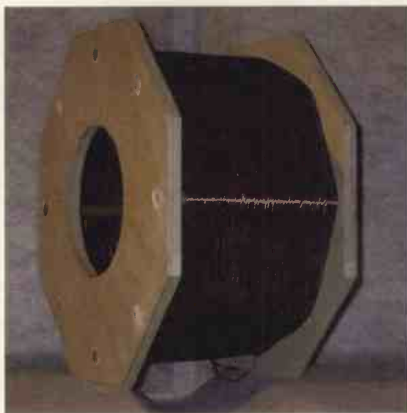
Fig. 8. Final load inductor – 3mH, with a Q of 600 at 136kHz.
