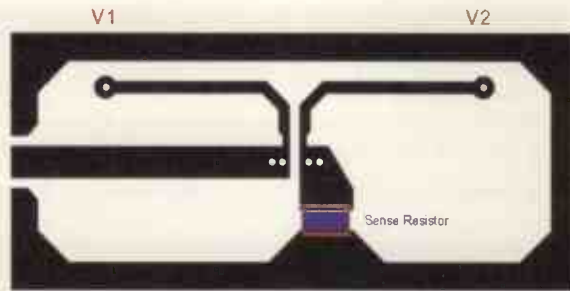
Fig. 5. The revised printed board pattern used for my prototype |Z| meter. Notice the additional dummy pads at U_2 and U_5 to equalise board capacitances between the two channels. Also note the guard tracks around sensitive pins of U_1 . Together with mirror imaging of tracks, these measures overcame the phase difficulty of my original board.
