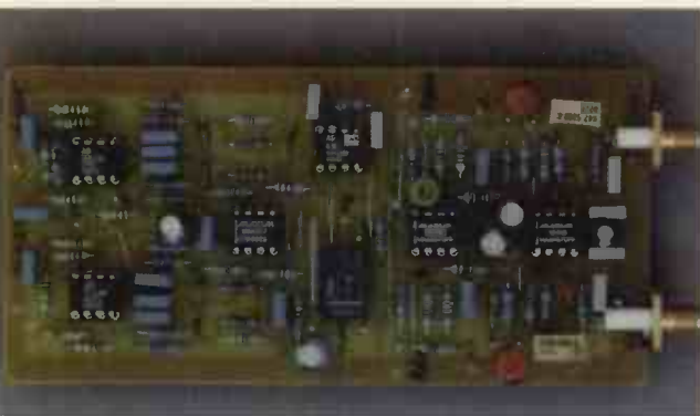
Fig. 8. Assembled |Z| meter printed board with two SMA connectors arranged to directly accept the test jig. By switching the central relay, the board can be made to operate in either measurement mode. The AD830 IC mounted near the relay, provides excellent common-mode rejection for differential measurements. To provide direct impedance measurement with 0.4995\Omega sense 'R', gain increasing resistors for V(2) output are fitted next to U_5 .
