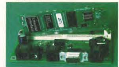
Java on a stick. This tiny Java controller with networking and Internet capability costs just $50. Les Hughes describes how to use it on page 531.
