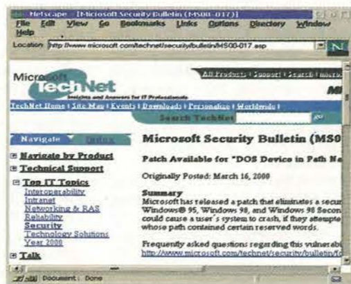
A new twist on web e-mail based bugs. If a Windows computer is forced into processing certain reserved DOS keywords, it crashes displaying a blue screen.
