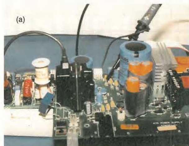
Fig. 5. Power supply and video drive assembly under test. The supply is a flyback converter and the line-output transformer in the centre of the picture is another flyback converter. In a), the 10:1 probe is reasonably well positioned, but in b) it is too close to the line-output transformer. The best solution is to solder a coaxial cable on the underside of the board, c).
