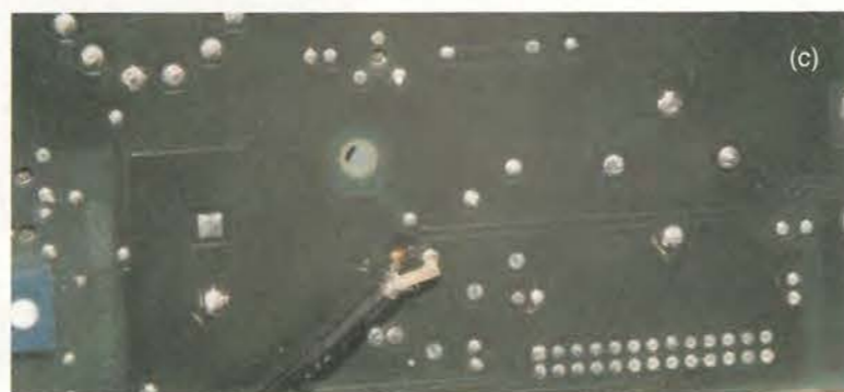
Fig. 5. Power supply and video drive assembly under test. The supply is a flyback converter and the line-output transformer in the centre of the picture is another flyback converter. In a), the 10:1 probe is reasonably well positioned, but in b) it is too close to the line-output transformer. The best solution is to solder a coaxial cable on the underside of the board, c).
