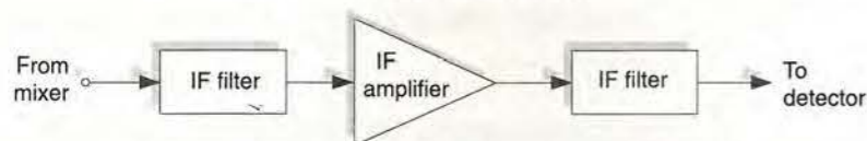
Fig. 1. Intermediate-frequency filtering arrangement, as used in a typical superheterodyne receiver.
