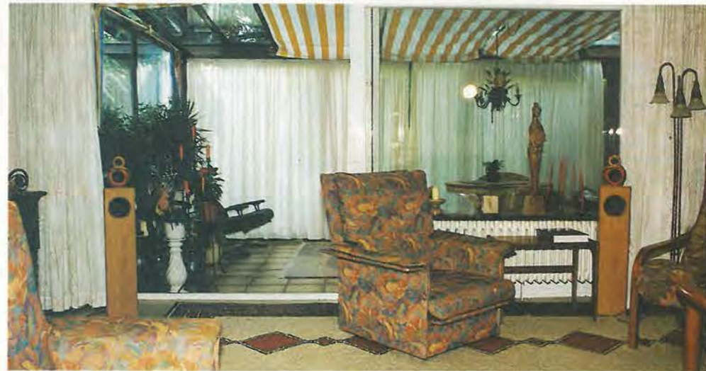
Fig. 11a). The boxes stand before the windows at a distance of 3.3m. They radiate into an acoustically-damped living-room. With a total height of 100cm and a width of 19.5cm they are well suited to the living-room, as you can see.
