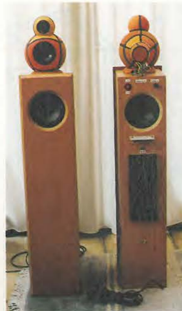
Fig. 9. Both faces of the cabinets are smart. The 5.5in 60W mini-woofer sets the width at 19cm (by 82cm by 23cm) of the bass enclosure. The spheres have a diameter of 15cm and 7.5cm.
