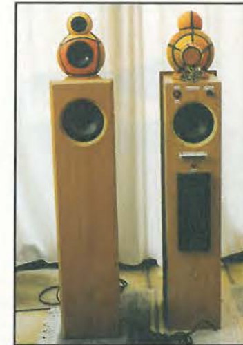
Features of the adaptable loudspeaker design on page 105 are a squarewave-in, squarewave-out active crossover, electronic bass roll-off compensation and spherical enclosures for minimal diffraction.
