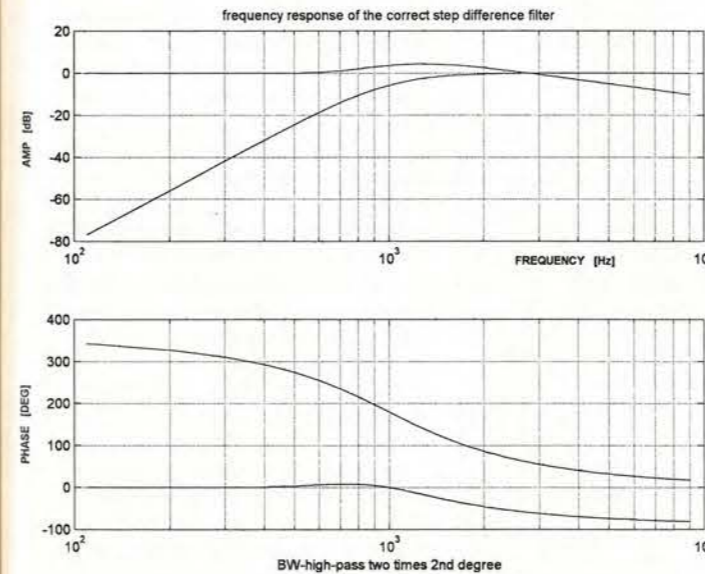
Fig. 4b). Amplitude and phase response of the high-pass section are standard. The response of the low-pass channel is for illustration purposes only. Response roll-off is poor, at only 6dB/oct independent of the order and character of the used filter.
