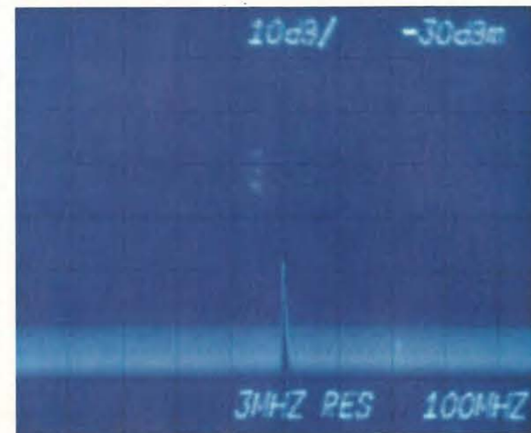
Fig. 1. An output stage oscillation on a faulty DC-300MHz amplifier, measured using a conventional 10:1 probe on a Tektronix 7603 frame with a 7L12 spectrum analyser plug-in. Top of the screen is -30dBm and the frequency of the oscillation is 1170MHz. This oscillation could not be seen on a 400MHz Tektronix 2465B real-time scope.
