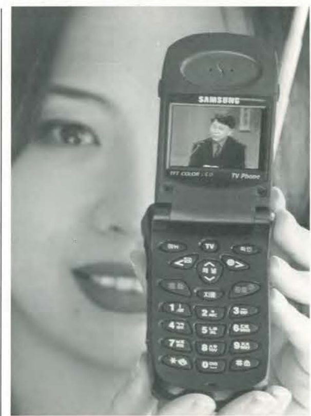
TV on the Radio... A combined television and mobile phone has been developed by Samsung Electronics. The company mounted a 1.8in LCD on the mobile hand-set and built in a miniature TV receiver. Talk time of the phone is claimed to be 170 minutes, while in TV mode the batteries last for 200 minutes, the firm said. The TV/phone will be available in Korea early next year.
