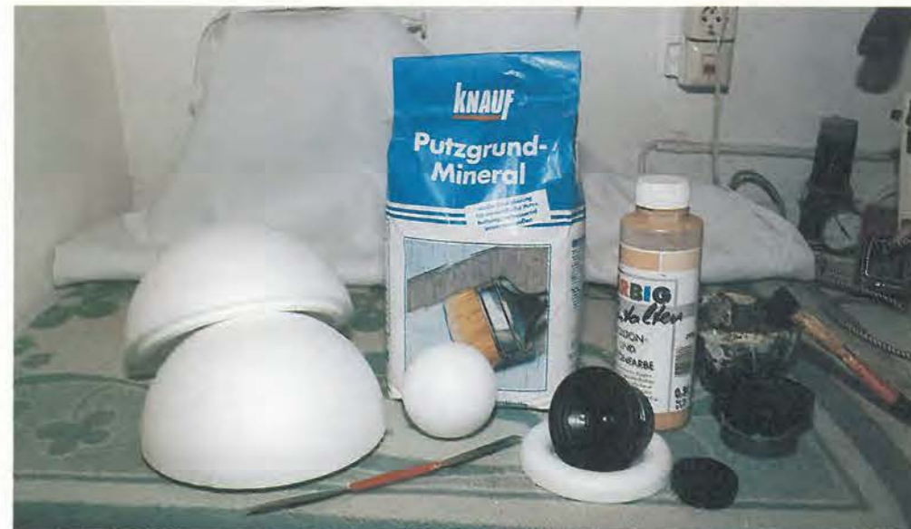
Fig. 8. This is the inexpensive material-mix to build the spherical boxes. The styropor spheres are an optimal acoustical solution as the styropor damps well and the sphere is the optimal form for radiating sound. The soft surface can be stabilised with ordinary papier mâché. If you coat all this with mineral material you get an attractive enclosure.
