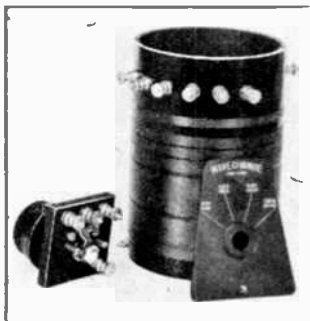
The Saxon tuner reviewed in these columns. Note the separate wave-change switch and indicator.
