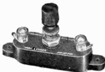
Vary Condenser. —Reversible terminals allow for mounting on panel or baseboard. Unique locking device enables capacity to be fixed as required. Two models are available. Maximum capacity, .0003. Maximum capacity, .001. Price 2/- each.
