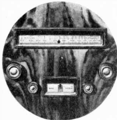
The latest in American control panels. The tuning scale is rectangular and horizontal, a pointer moving along it as the control is altered. Below it is the tone control dial, marked "bass" and "treble," also with a moving pointer.
