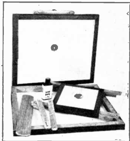
A view of the set of parts for building the "Kone Dope" linen diaphragm speaker chassis. A completed chassis is at the back.
