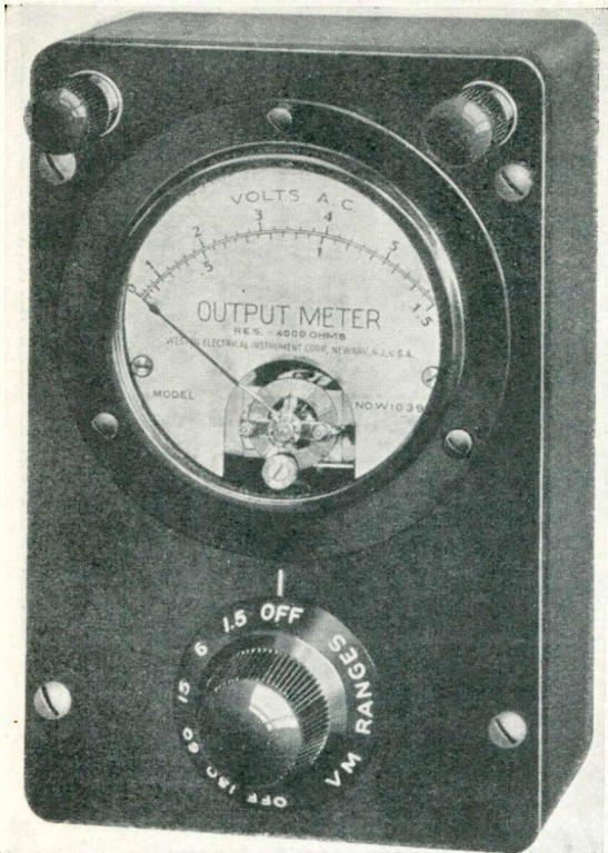
A good output meter enables a great variety of advanced test and experimental work to be done, especially when used in conjunction with a modulated high-frequency oscillator such as that which has been specially designed for readers of this section by Mr. Tyers for publication in an early issue
