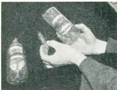
Electron multiplier tubes developed by the Farnsworth Television Company of America. These tubes have no filament and give an amplification up to a million times
