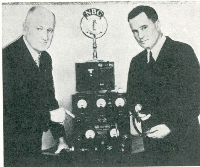
Major General James Harbord, Chairman of the Radio Corporation of America (left) and R. C. Patterson, jun., of the N.B.C., inspecting the tiny R.C.A.-Victor short-wave receiver and transmitter used by Captain Stevens and Captain Anderson on their recent stratosphere flight. The receiver weighs 15 lb. and the transmitter only 40 lb.
