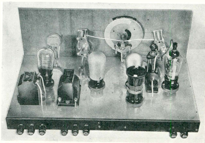
The general arrangement of the A.C. Standard Short-waver resembles that of the battery model: the layout on the top side of the chassis remains unaltered except that five-pin valve holders have been fitted
