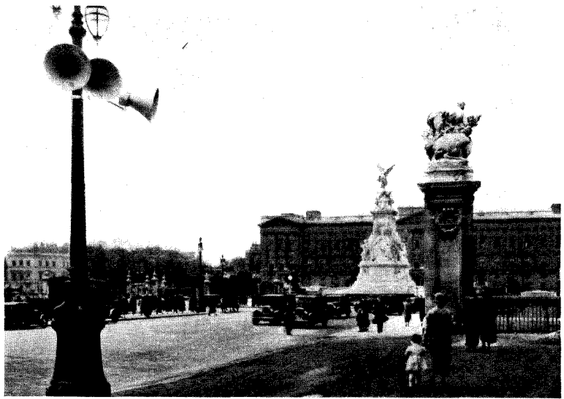
For public-address work the high efficiency of the horn-type loudspeaker constitutes an important advantage. It is even more directional than the open baffle type, however, and so must be placed carefully to cover the desired area
