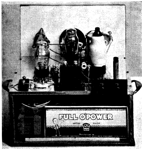
The batteries fit neatly in the lower compartment. Note the carrying handles fitted to the ends of the set
