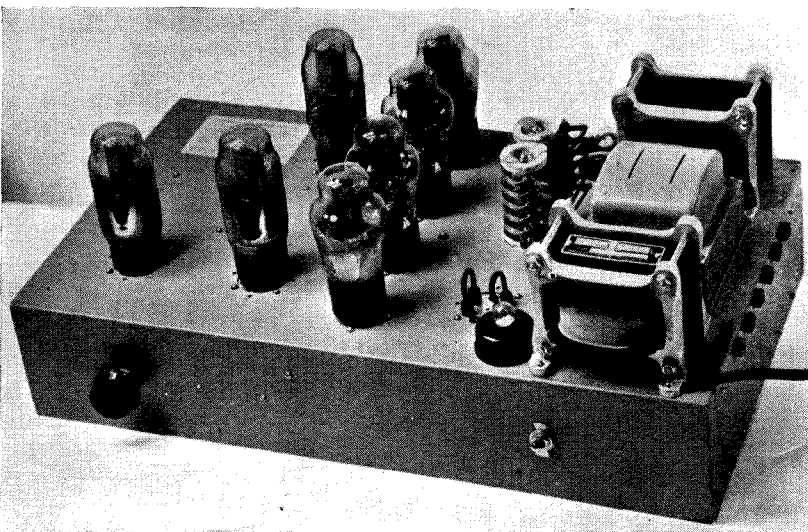
An A.C./D.C. amplifier which gives an undistorted output of nearly 12 watts made by Universal High-voltage Radio, Ltd. It uses Ostur-Ganz valves and costs £21
