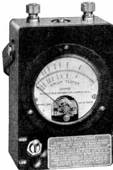
The model 563 circuit tester made by the Weston Electrical Corp., Ltd. Its use is to enable the resistance in a circuit to be ascertained easily
