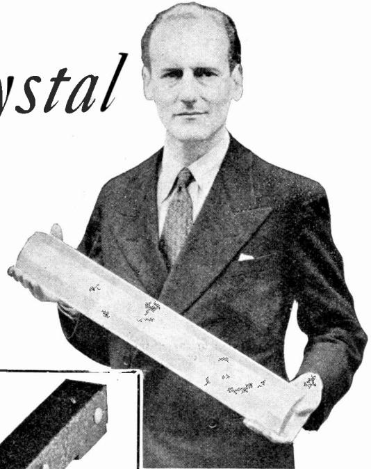
Rochelle salt in the raw! An American engineer is holding a crystal of glass-like transparency. There is enough crystal here, when cut, to develop 1,500 volts
