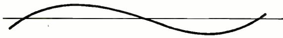
Fig. 2(b).—The audio frequency, in this case 50 per cent of the carrier amplitude
