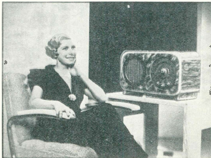
Cabinets, too, have advanced in design! This photograph shows a new Ekco super-het with moving-coil loud-speaker housed in an all-bakelite cabinet. The large dial is a help for accurate station-getting
