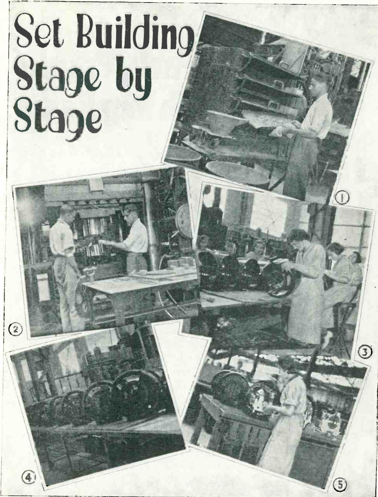
Our photographer recently paid a visit to the huge radio works of E. K. Cole, Ltd., at Scuthend-on-Sea. He brought back this set of pictures showing how Ekco's famous bakelite cabinets are made. (1) Measuring out an appropriate amount of powder to make one cabinet. (2) Taking the "cooked" mould out of the press. (3) Polishing the finished cabinets. (4) Cabinets passing to the assembly benches on an endless belt. (5) Putting an Ekco set chassis in an Ekco bakelite cabinet.
