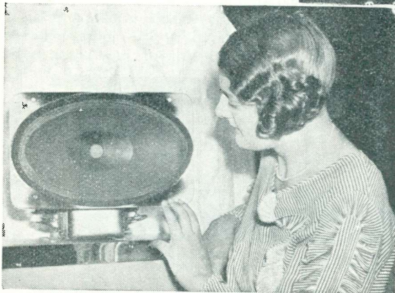
A new loud-speaker by H.M.V., and used in many of their sets, has two cones, one of metal and one of parchment, and is oval in shape to ensure good frequency response
