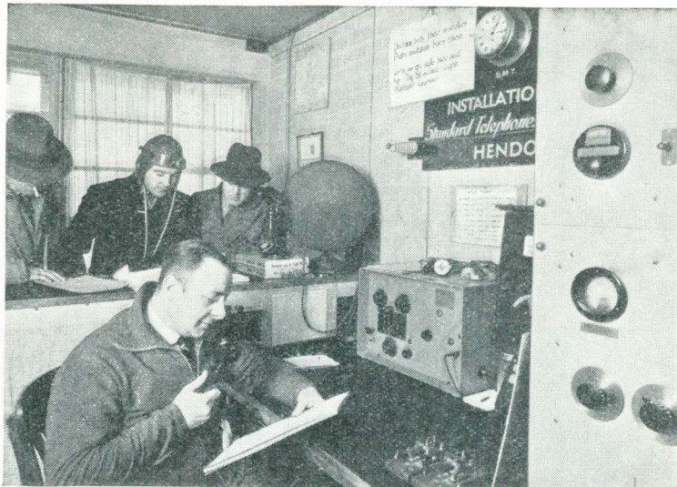
This is the transmitter at Heston Airport, from which you can pick up weather reports throughout the day on 1,202 metres
