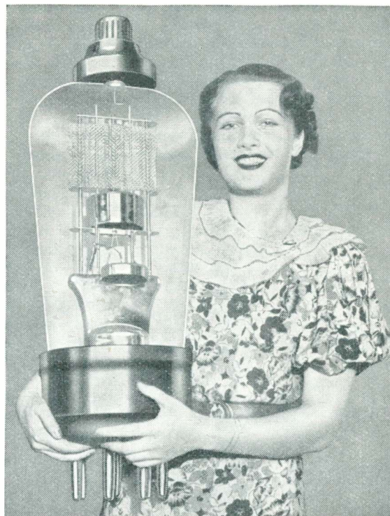
The author suggests that you use a screen-grid valve as a diode detector—something on the lines of this G.E.C. model.
