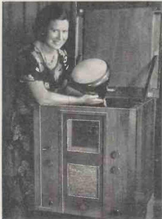
Photo courtesy Telefunken The Telefunken cathode-ray receiver for the home. It is expected that this type will shortly be available for the reception of the Berlin short-wave transmissions which are expected to commence in the autumn.
