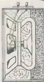
The top drawing shows clearly how the plywood is cut to make the case for housing the midget moving-coil loud-speaker. On the left you see how the loud-speaker is wedged into its case with a rubber sponge, the remaining space being filled with slag-wool or ordinary cotton wool
