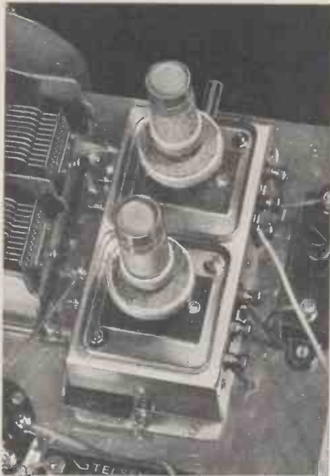
HEART OF THE SET No doubt a deal of the set's efficiency is due to the iron-core coils, which are shown here with the screening cans removed
