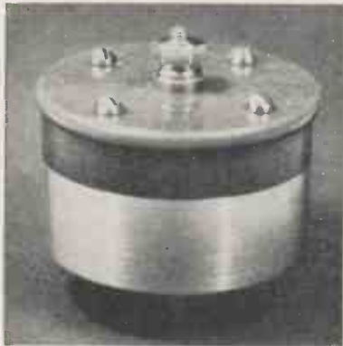
MOUNTED QUARTZ CRYSTAL This shows the Brookes quartz crystal. It has been specially designed for this set
