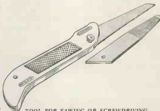
TOOL FOR SAWING OR SCREWDRIVING Fig. 1.—The Eclipse tool fixed up for sawing. The screwdriver blade fits into the other end
