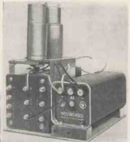
SEPARATE MAINS PACK The mains unit is built separately and fits snugly in the cabinet between the set chassis and loud-speaker
