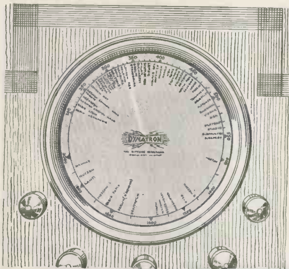
A REALLY "HOT" DIAL The Dynatron dial—by Hacker of Maidenhead. A neon beam is the only movable part. The width of the beam varies according to the setting of the selectivity switch in the set
