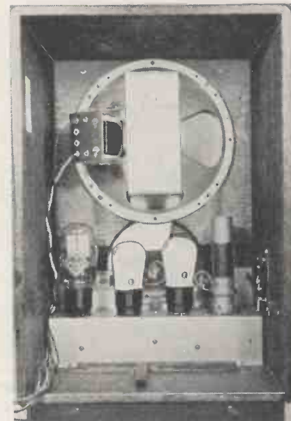
"The neat chassis and layout. All the small components are mounted out of sight"
