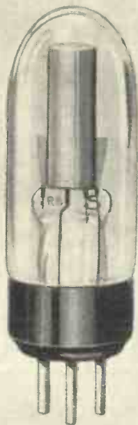
A crater lamp as used for television. The emission is from a small hole at the end of the cylinder
