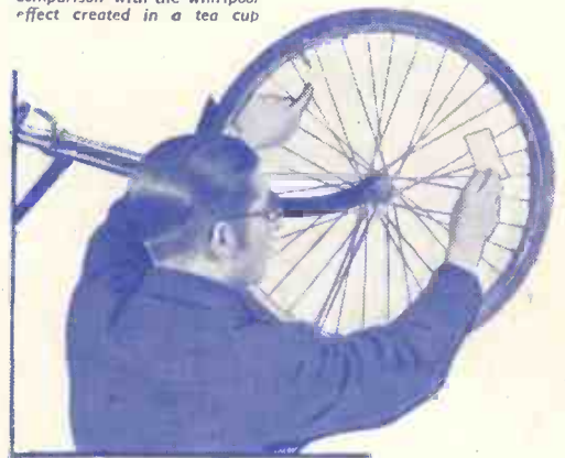
A card held against a rotating bicycle wheel produces a pitch which varies with the speed of the wheel, illustrating note frequency
