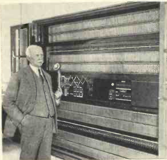
This huge public address system, installed in an American school at St. Louis, makes it possible for the school superintendent to broadcast messages to the 3,000 pupils, either simultaneously or in sections
