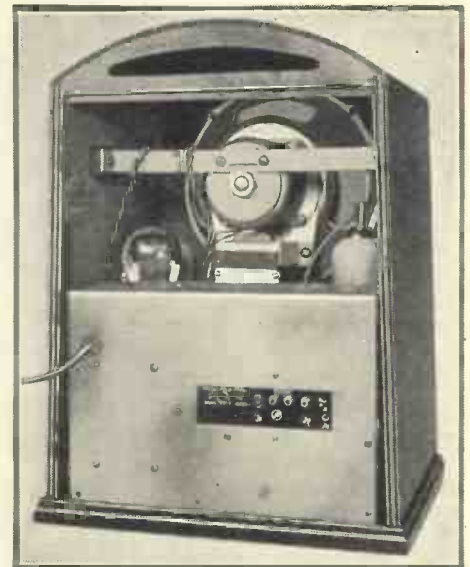
"Set chassis is of unusual design, being built up at the back to give protection to the valves"
