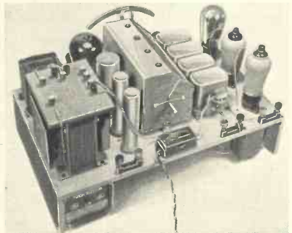
LOOKING FROM THE BACK The arrangement of the components on the top side of the baseboard can be seen from this photograph. Note the fuses behind the ganged condenser
