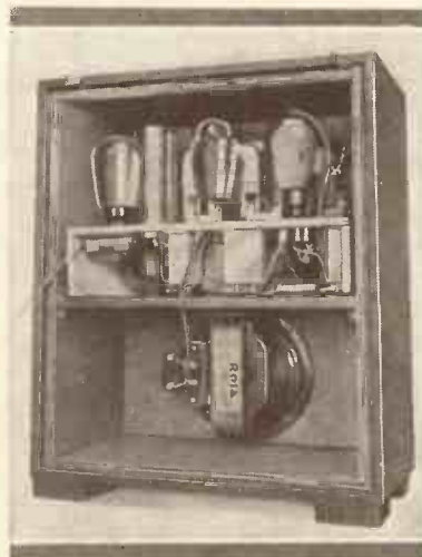
MODERN CHASSIS DESIGN The set itself is mounted on the removable aerial framework for easy assembly and manipulation
