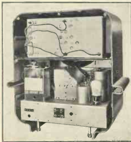
"The high-tension battery . . . fits snugly on a shelf behind the loud-speaker. Room has been made for the 2-volt accumulator in one corner"
