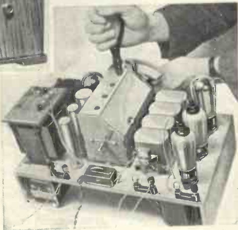
GANGING THE SET Although there are four trimmers on the condenser the ganging is quite simple if carried out in the right way
