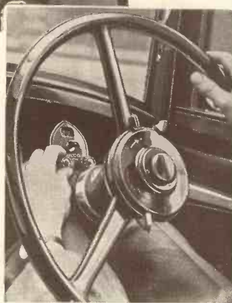
To cut out interference from the electrical system of a car, suppressor resistances must be fitted in series with each plug lead as shown in the photograph above. Car radio sets are simple to control and the right-hand photograph shows the control panel of a Philco-fitted car
