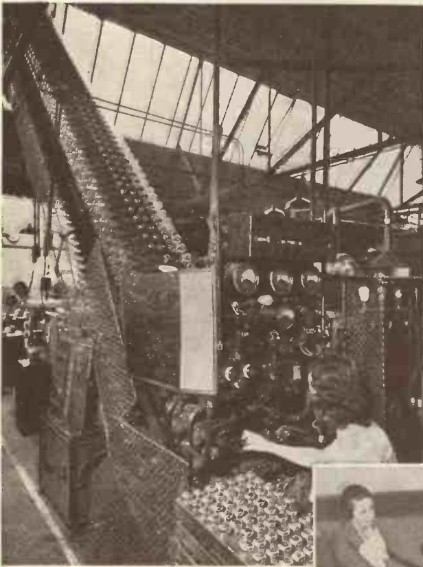
AMAZING VALVE MACHINE This robot machine in the Cossor works "getters" valves and then runs them with grid and anode voltage to stabilise the characteristics
