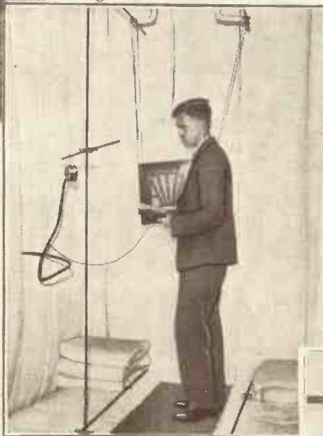
This is where loud-speakers are tested. This room is padded to a depth of 18 in. with wool to obviate any possibility of sound reflection. On the right you see the apparatus for testing lightning arrestors. It can generate 250,000 volts!
