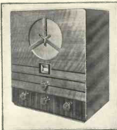
"Mr. Murphy has combined the excellent selectivity of the super-het with the good volume and quality obtainable from class-B to produce a notable battery set"
