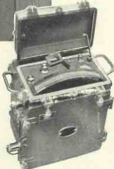
(Above) A Marconi Echometer installed on the bridge, and (right) the Echo-scope for investigating the sea-bottom
