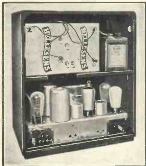
"Briefly, the circuit consists of five valves in super-het sequence with one stage of intermediate-frequency amplification." A pentode is used as a combined oscillator and first detector
