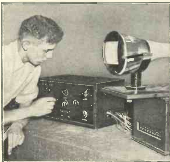
CATHODE-RAY TUBE CHECKING In commercial-set tests a cathode-ray tube with a suitable time base gives an accurate picture of the set output and enables the ganging to be accurately done
