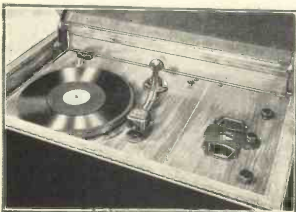
". . . all the controls, with the exception of the volume control, are mounted on the motor-board to the right of the gramophone turntable."
