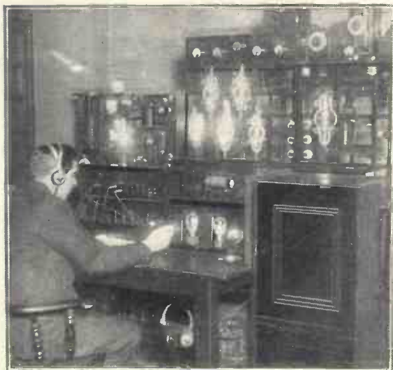
A RADIO RELAY At the controls of the Sheffield relay station, which puts broadcast programmes over a landline. No high-frequency carrier is used
