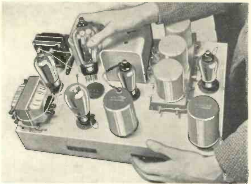
ALL READY TO TRY THE SET OUT—PUTTING THE VALVES INTO POSITION
