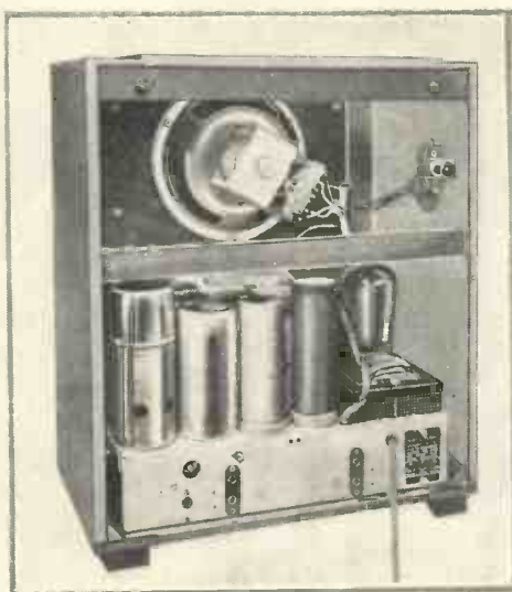
"The makers have followed the conventional idea of a set built up on a metal chassis and fixed at the bottom of the cabinet."
