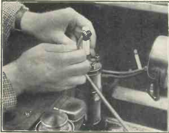
Putting the final touch to interference prevention in a car—the main distributor resistance being connected in the ignition system
