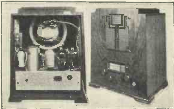
NEW FOUR-VALVE A.C. SUPER-HET A handsome walnut cabinet houses the new Marconiphone A.C. super-het. Note the easily-read tuning scale in the right-hand photograph
