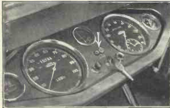
This Rotax system, typical of that fitted to many cars, has provision on the fascia board for a plug which can be connected to the low-tension side of the set
