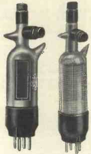
LIGHT-SENSITIVE CELLS Two Osram photo-electric cells. That on the left is the type KMV6 or CMV6; the electrode system can be clearly seen in the right-hand photograph
