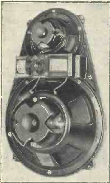
DUAL LOUD-SPEAKERS The Celestion Reetone assembly consists of two moving-coil reproducers mounted one above the other
