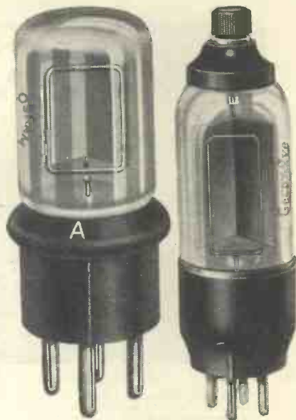
MAKING LIGHT DO WORK With such cells as these (Osram KG7 on left and the Gecovalve on the right) light can be made to do useful work
