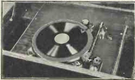
VIEW OF THE MOTORBOARD This photograph shows how the motorboard of the D.C. Calibrator is arranged. The motor will work from either D.C. or A.C. mains
