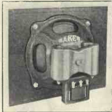
NEW LOUD-SPEAKER A new Baker instrument designed for sets with a class-B output stage
